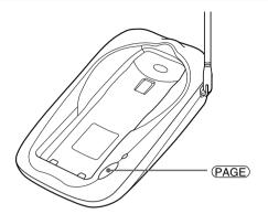
To locate the handset while it is off the base, press (PAGE). The handset beeps for 60 seconds.
